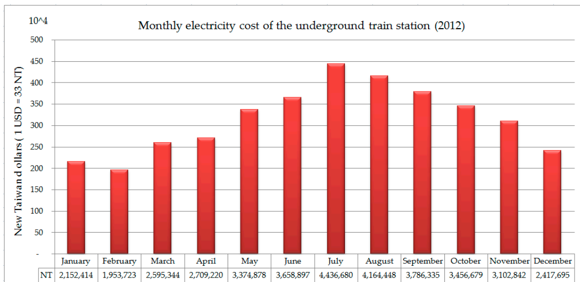
Figure 4. Monthly electricity cost of the underground train station in 2012.
