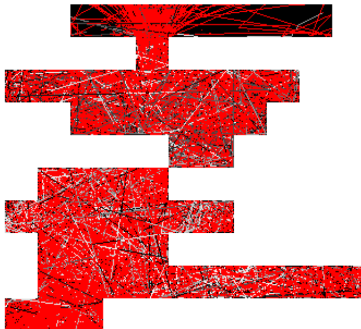
Figure 1. At the top of the oil productive layer (the black rectangle), the flow connectivity/tortuosity can be measured and visualized by the Brownian motion model. The clear tree-like oil flow pattern is observed on the well scale.
