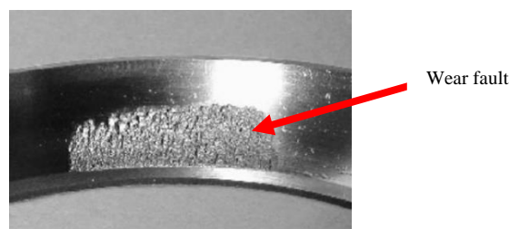
Figure 8. Bearing outer ring wear fault.
