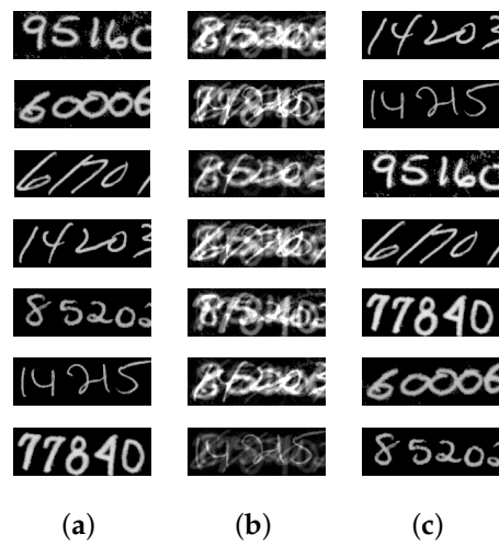
Figure 8. Mixing and unmixing of zip codes. (a) Original; (b) Mixture; (c) Recovered.
