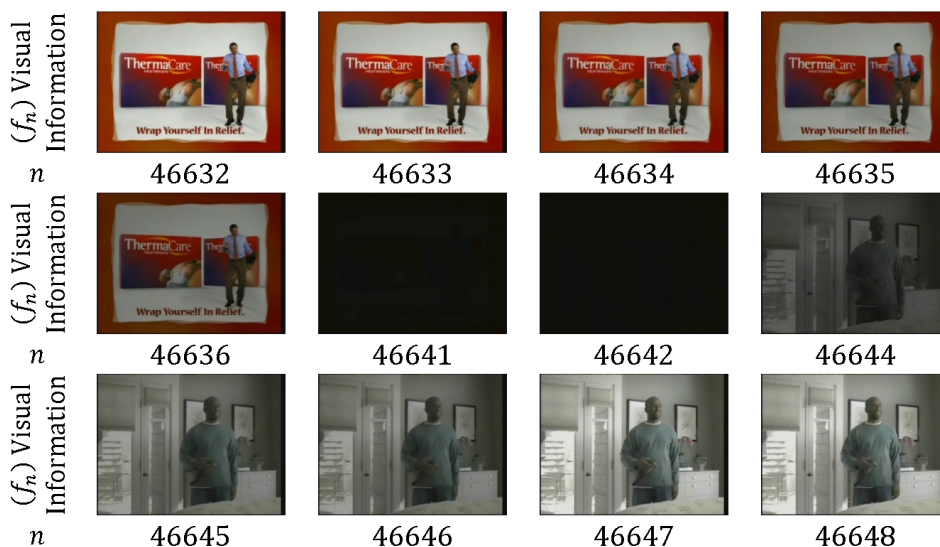
Figure 10. Fade out-in transition example with 15 frames involved in transition ( n = 46,632-46,648 ). Frames are extracted from TRECVID 2005, Video ID: 02-20041106_110000_MSNBC_MSNBC.
