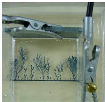
Figure 2. Experimental setup. The Zn fractal trees originate at the thin graphite cathode seen at the bottom, and grow toward the thick Zn anode. The applied voltage is 9.5 V.
