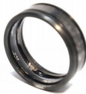
Figure 24. Photo of failed bearing (outer ring worn).
