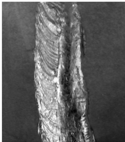
Figure 1. Laboratory sample of an OK weld.
