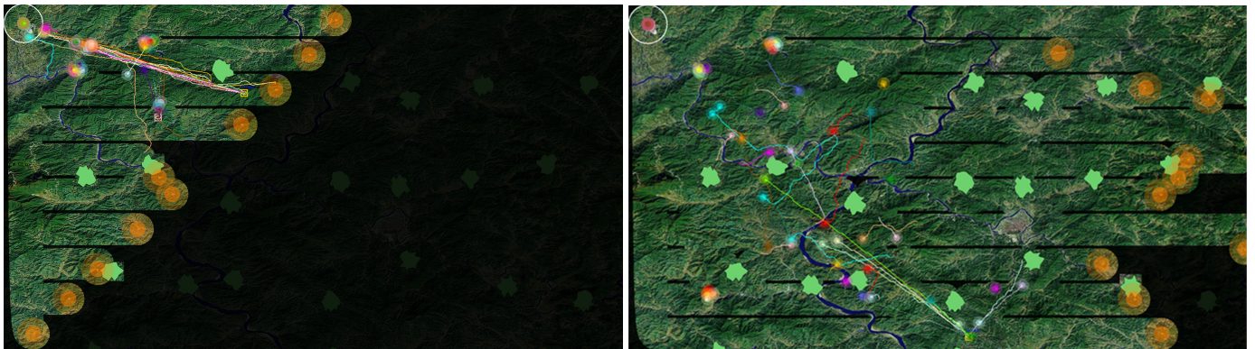
Figure 8. Simulation screen shots. On the left is a few moments after simulation started, when the victims found are rescued by appropriate robots. Towards the end (right), as the search area reduces drastically, some of the search robots started returning to the base while the rescue is ongoing.
