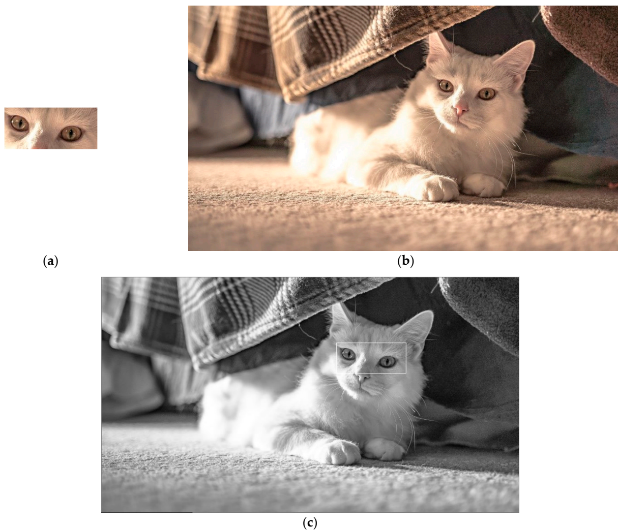
Figure 7. (a) Predefined template image ( 160 \times 70 ); (b) source image ( 960 \times 540 ); (c) TM result.
