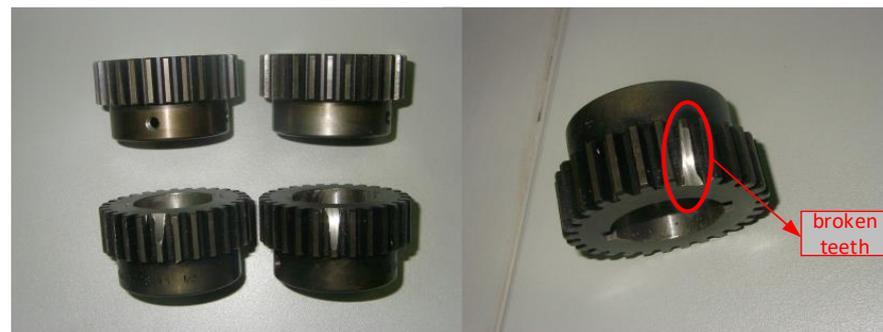
**Figure 20.** Broken-teeth-seeded planet gear.
