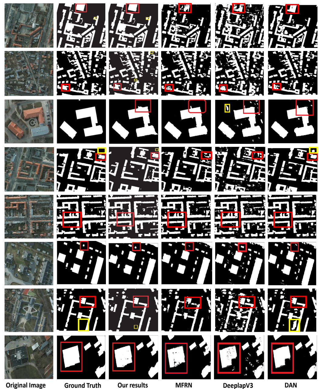
Figure 3. The building’s segmentation on Potsdam dataset. From left to right: original image, ground truth, our results, the multiple-feature reuse network (MFRN), Deeplap-V3, and the dense-attention network (DAN). The red boxes indicate improvement, while the yellow boxes indicate a false classification.
