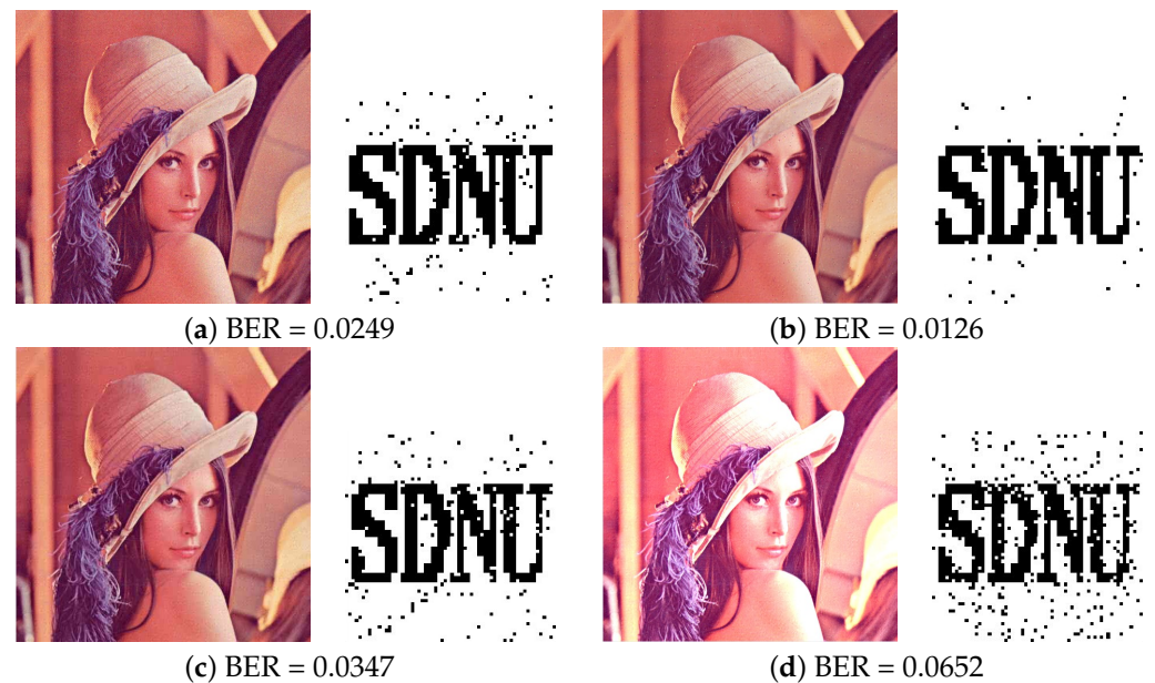
Figure 9. Results under different types of attacks and recovered watermark from Lena image (a) Gaussian Noise (var=0.0015) (b) Salt and Pepper noise (density=0.0015) (c) JPEG compression (Q = 30) (d) Amplitude Scaling 1.5.
