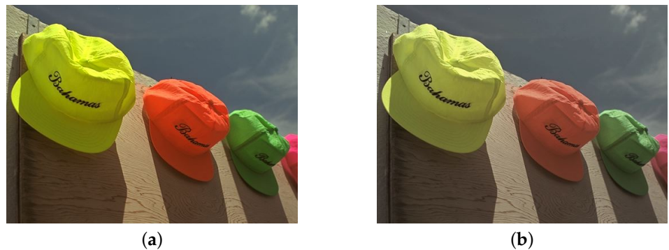
Figure 2. Image comparisons of colorfulness metrics. (a) Reference image with colorfulness is 0.9462; (b) Chrominance distortion image with colorfulness is 0.4563
