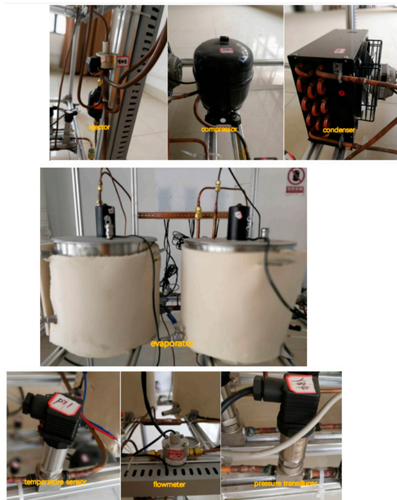
Figure 4. Components of the multi-evaporator refrigeration system.
