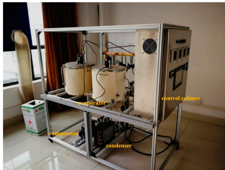
Figure 3. Experimental platform of the multi-evaporator refrigeration system.
