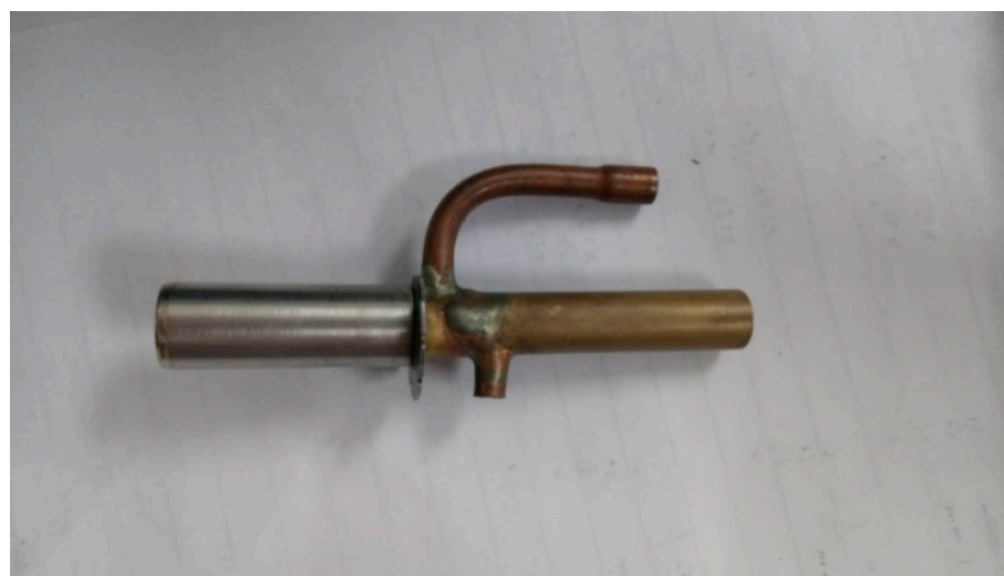
Figure 5. The external view of the welded EEV-based ejector.
