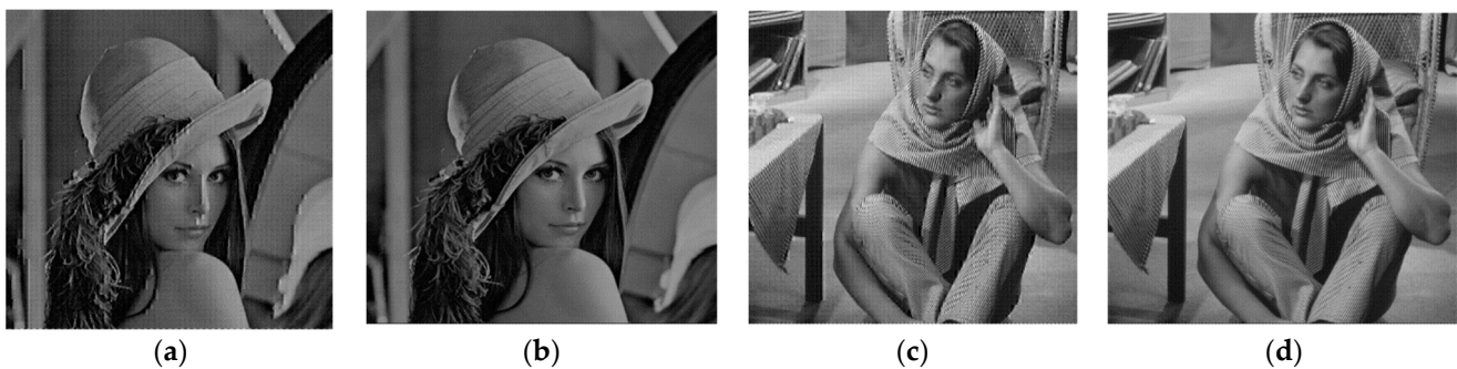
Figure 7. Results of compression for the 512 \times 512 grayscale images of Lena and Barbara. (a) Lena image reconstruction using DWT with PSNR = 29.9001 dB and rate (bpp) = 3.2855; (b) Lena image reconstruction using the proposed method with PSNR = 34.7809 dB and rate (bpp) = 1.8158; (c) Barbara image reconstruction using DWT with PSNR = 27.7496 dB and rate (bpp) = 3.7896; (d) Barbara image reconstruction using the proposed method with PSNR = 33.3092 dB and rate (bpp) = 1.9806.
