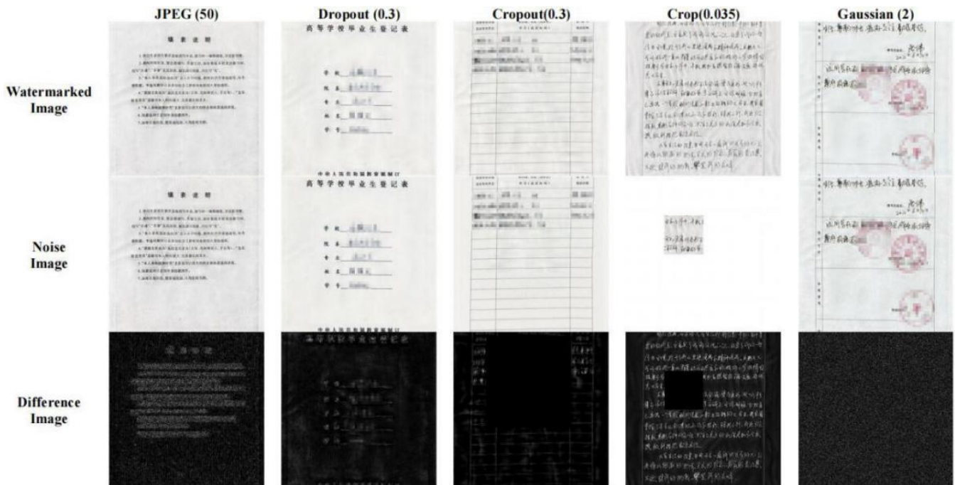
Figure 10. Watermarked archives image after noise attack and its residual image.
