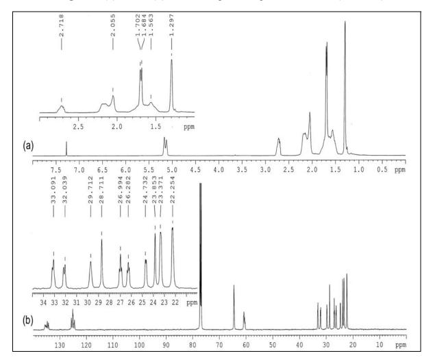
Figure 3. JRES spectra of purified ENR-50 (in CDCl<sub>3</sub>).
