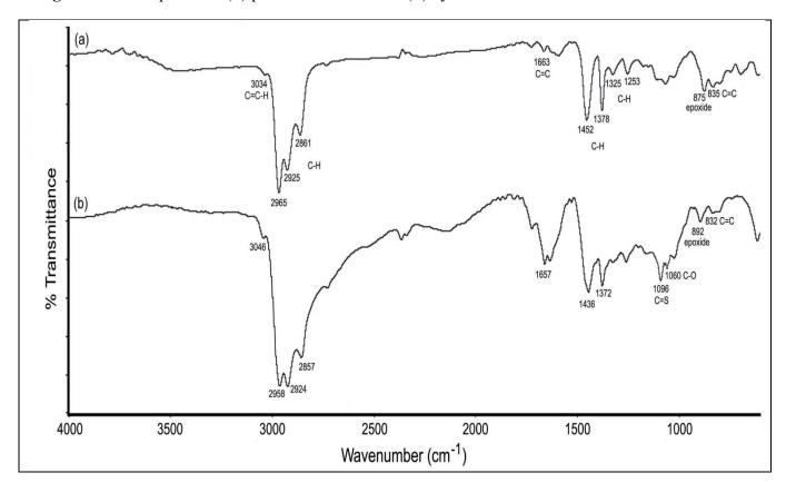
Figure 7. FTIR spectra of (a) purified ENR-50 and (b) cyclic dithiocarbonate derivative of ENR-50.
