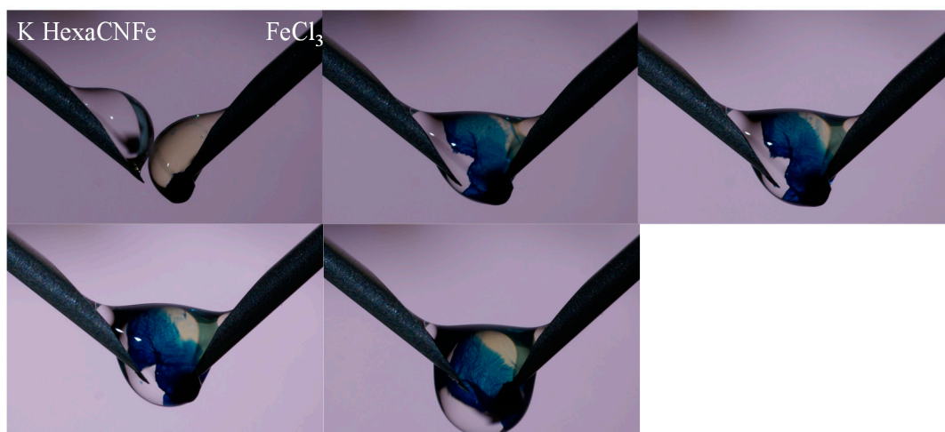
Figure 1. “In-drop” synthesis of Prussian Blue.
