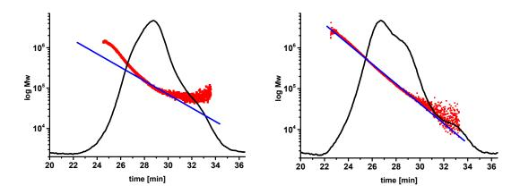
**Figure 2.** SEC-MALLS chromatograms of the same sample dissolved individually. The chromatogram on the left shows a poor state of dissolution; the chromatogram on the right depicts a satisfactory state of dissolution of the polymer. The red dots represent a light scattering signal; the blue lines represent a fitted (linearized) light scattering signal [34].
