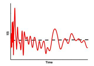
**Figure 3.** The fluctuation of scattered light over time (in the range of milliseconds). The dotted line represents the SLS-signal and the red line represents the DLS-signal.
