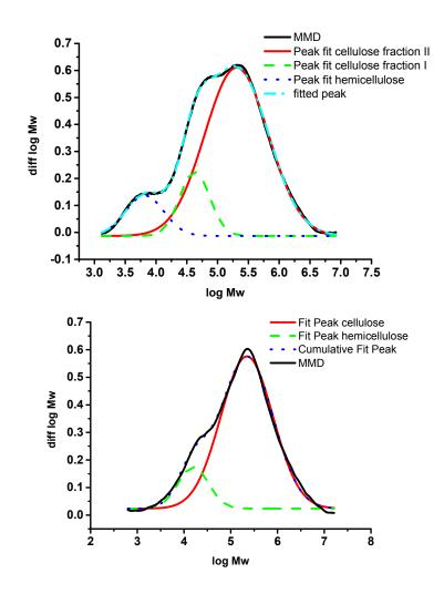
**Figure 5.** MWD of a hardwood pulp (**top**) and a softwood pulp (**bottom**) with multiple-peak fits of the cellulose and hemicellulose fraction [34].
