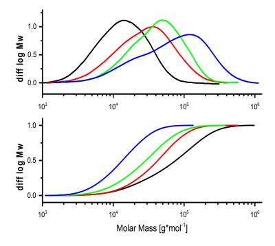
**Figure 4.** Differential (top) *vs.* cumulative distribution of molar mass (cellulose degradation kinetics).
