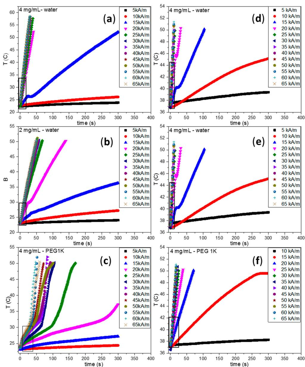
**Figure S3.** Heating curves of small  $\text{Fe}_3\text{O}_4$  MNPs dispersed in different media and recorded starting with room temperatures (left panels: a–c) and 37 °C (right panels: d–f) as a function of AC magnetic field amplitudes at 355 kHz. The black rectangles frame the slope ( $\Delta T/\Delta t$ ) used in SAR determination.
