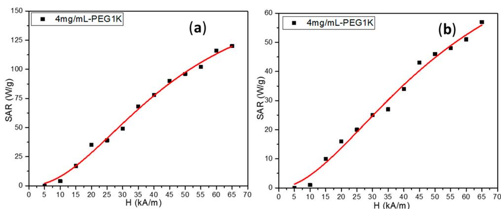
**Figure S5.** SAR values of  $\text{Fe}_3\text{O}_4$  MNPs synthesized in (a) PEG 200 and (b) EG as a function of AC field amplitudes and at a frequency of 355 kHz. The  $\text{Fe}_3\text{O}_4$  MNPs are dispersed in soft solid PEG1000 and the hyperthermia measurements have been performed starting with room temperature up to 37 °C. The data are fitted with a sigmoidal function (red lines).
