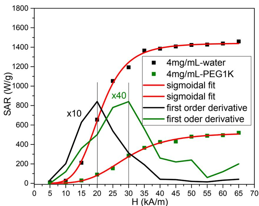
**Figure S6.** The SAR values of small  $\text{Fe}_3\text{O}_4$  MNPs as a function of AC field amplitudes in water and PEG1K. The experimental results have been fitted with a sigmoidal function (red lines). The first-order derivatives of the experimental data were multiplied by 10 and 40 for clarity (black and green lines). The maxima in first-order derivative correspond to the inflection points of sigmoidal function and give the values of  $H_{\text{CHyp}}$ .
