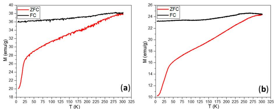
**Figure S2.** ZFC and FC magnetization curves of (a) small and (b) large  $\text{Fe}_3\text{O}_4$  MNPs, acquired in an external magnetic field of 50 mT.
