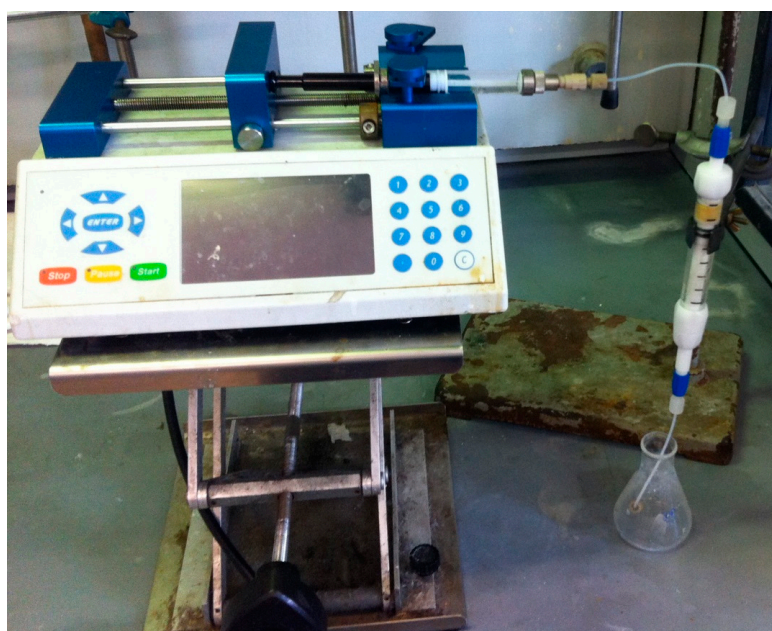
Figure S1. Set-up of continuous flow experiment;
