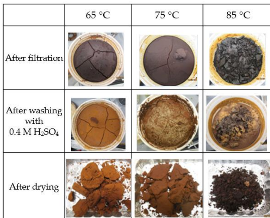
Figure 8. Contrast in lignin colour when precipitated at different 65, 75 and 85 °C.
