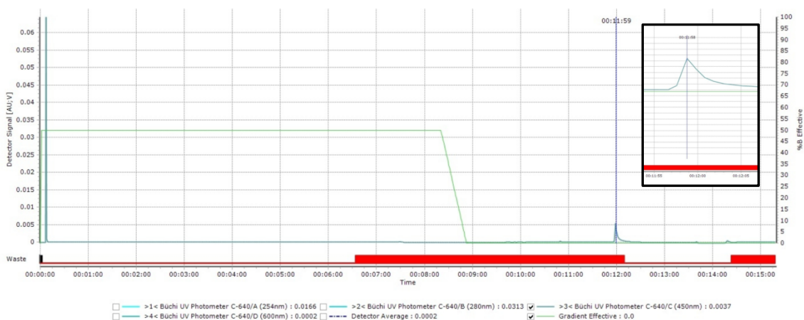
Figure S25: MPLC purity assessment for compound 3a *** (time~12 min). A gradient of acetonitrile in water followed by THF was applied.
