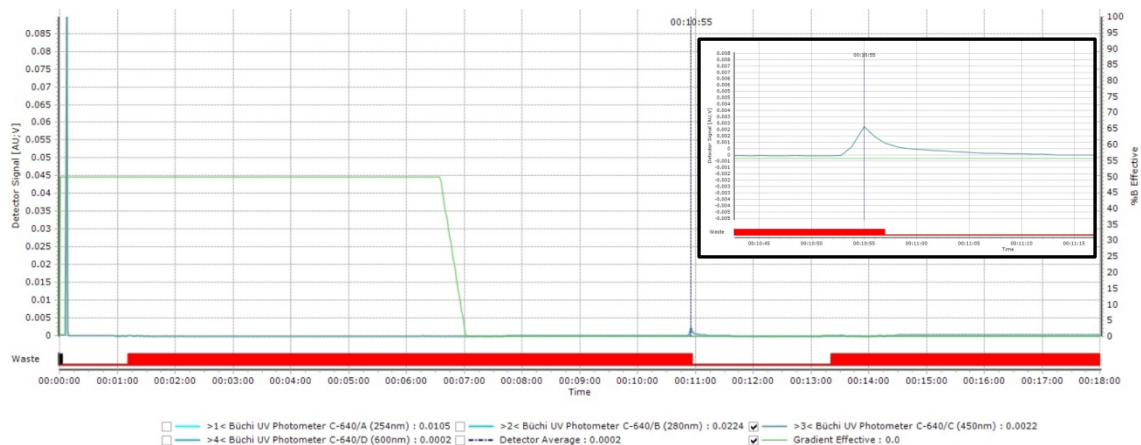
Figure S22: MPLC purity assessment for compound 2b •• (time~11 min). A gradient of acetonitrile in water followed by THF was applied.
