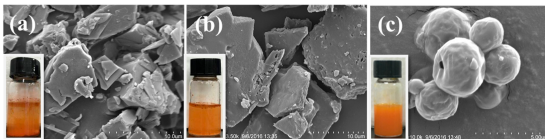
Figure 1. Appearance (dispersed in deionized water at a lutein concentration of 1 mg/mL) and SEM morphology images of native lutein (a); lutein-loaded-lecithin microcapsules (b) and lutein-loaded NaCas microcapsules (c).
