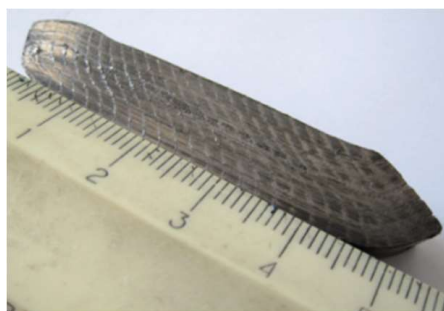
Figure 1. A picture of ECAP processed billet shows transformation of a reference square array drawn on the four 50 \times 10 mm faces at the initial state.
