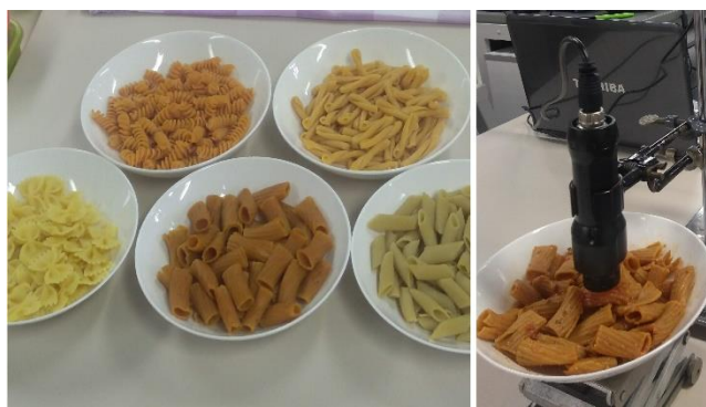
Figure 1. Different morphologies of the investigated pastas and a typical experimental set-up for the measurement of a pasta (here without sauce) with the handheld NIR spectrometer.
