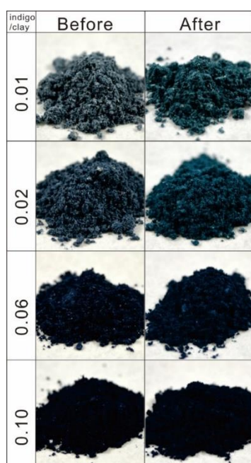
Figure S6. Coloration comparisons of the indigo–palygorskite mixtures with different ratios before and after heating.
