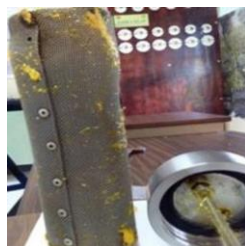
Figure 5. Perezone extraction with scCO 2 , the yellow crystals correspond to the isolated product.
