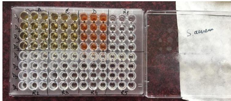
Figure 2. Minimum inhibitory concentrations (MICs) determined by a broth microdilution method for TMs (B, R6) and TMc (C, R7)
