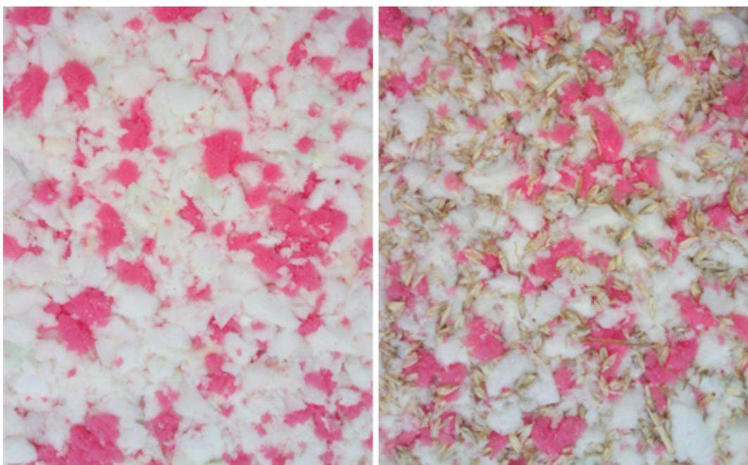
**Figure 1.** Surface view of the thermal insulation layer, board without husks on the **left**, board with addition of husks on the **right**.
