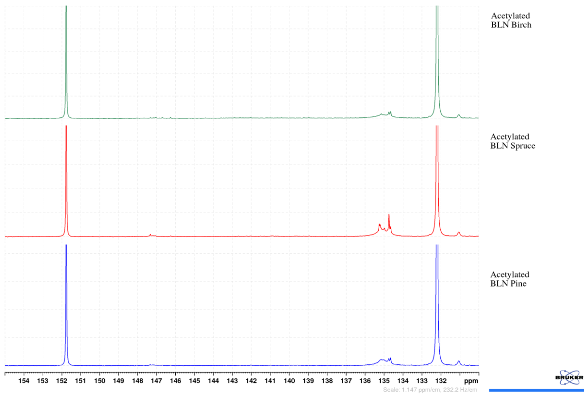
Figure S11. ^{31}\text{P} NMR of the acetylated lignin birch, spruce and pine
