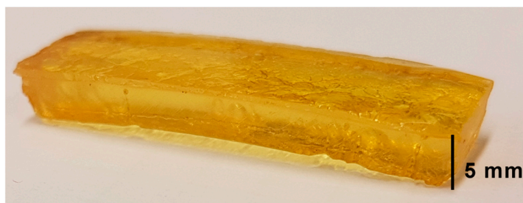
Figure S23. Cross-linking of 1 at 300 °C in a silicon form for 2 h, producing a hard, cross-linked PPE resin.
