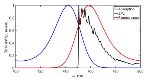
**Figure 7.** Calculated zero phonon line (ZPL), absorption, and fluorescence of F760 emitter. The shape of ZPL corresponds to the strong electron-phonon coupling. The inhomogeneous broadening is  $200 \text{ cm}^{-1}$ . The resulting Stokes shift is about 20 nm.
