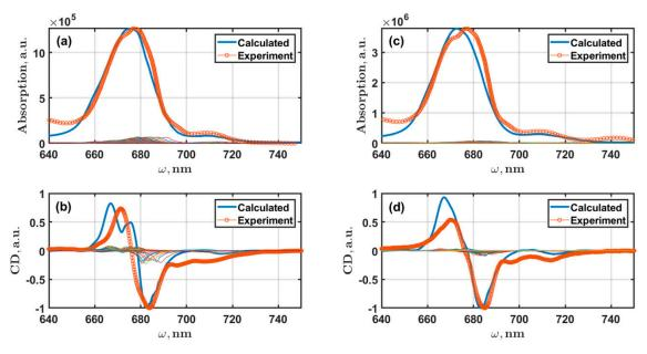
**Figure 5.** Calculated exciton absorption (upper plots) and CD (lower plots) spectra for PSI monomers (**a**,**b**) and trimers (**c**,**d**). The experimental absorption spectra measured at 4 K; CD spectra measured at 77 K. The absorption and CD spectra were modeled for the corresponding temperatures. FWHM of inhomogeneous broadening is  $200 \text{ cm}^{-1}$ . All data averaged over 1500 realizations of the Monte Carlo method. The thin colored lines are the intensities of exciton states.
