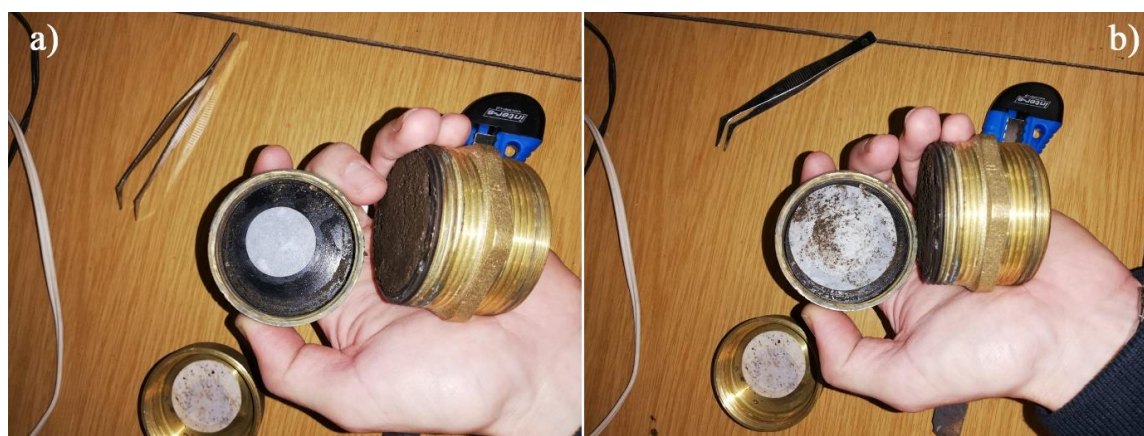
Figure 9. Application of the two concentric paper filters, with diameters of 30 mm (a) and 50 mm (b).
