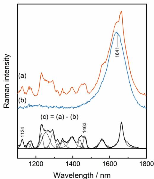
**Figure S2.** Construction of the difference spectrum (c) by subtracting the water spectrum (b) from the spectrum of the peptide in water (a), with indicated reference bands. The difference spectrum is fitted with Gaussian-Lorentzian shape components. The excitation wavelength is 325 nm.
