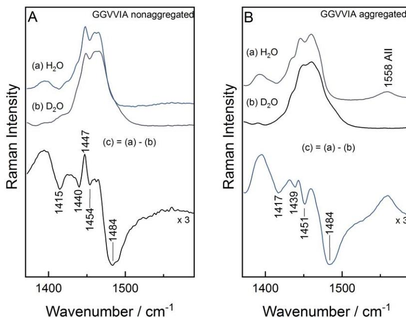
**Figure S1.** Raman spectra of nonaggregated (A), and aggregated (B) GGVVIA peptides in H<sub>2</sub>O (a), and D<sub>2</sub>O (b), as well as the difference spectra of H<sub>2</sub>O minus D<sub>2</sub>O (c). The spectra were collected using HyperFlux PRO Plus Raman spectrometer at 785 nm excitation.
