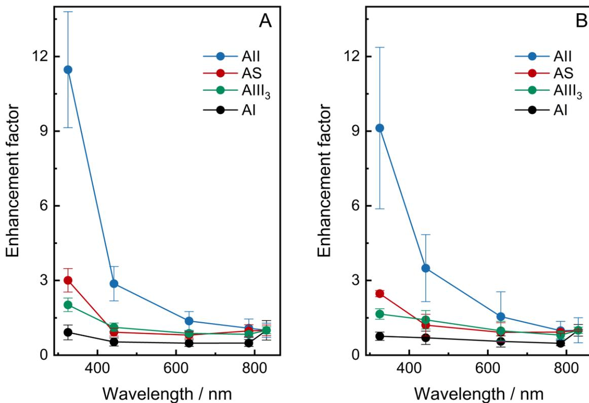
**Figure S3.** Wavelength-dependent enhancement factors for selected vibrational modes. The relative intensities for spectral bands were acquired with respect to the spectral band near 1124 cm<sup>-1</sup> (A) and the deformation vibration of water near 1641 cm<sup>-1</sup> (B).
