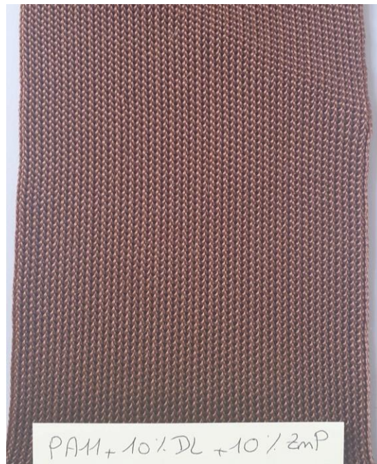
Figure S2. KL and ZnP filled PA11 knitted fabric structure.
