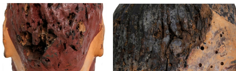
Figure 2. Wooden puppet heads (WPHs): deep deterioration of constitutive materials (left); flight holes 1.5–3 mm in diameter (right) related to the Anobium punctatum (de Geer 1774) infestation.
