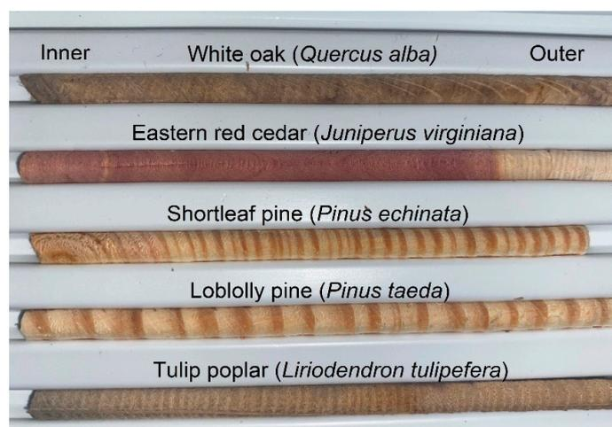
**Figure 4.** Example of tree cores collected with a 5-mm increment borer.
