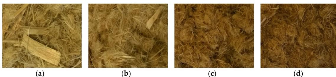
**Figure 7.** Morphology of spruce wood after steam refining using different treatment conditions [ $\log R_0$ ; °C; min]: (a) 2.47; 150; 10, (b) 3.06; 160; 20, (c) 3.36; 180; 10, (d) 3.95; 190; 20.
