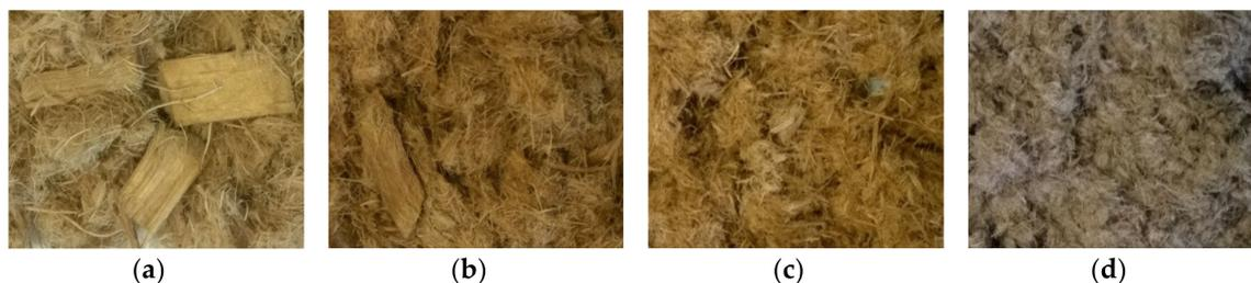
**Figure 6.** Morphology of poplar wood after steam refining using different treatment conditions [logR<sub>0</sub>; °C; min]: (a) 2.47; 150; 10, (b) 3.06; 160; 20, (c) 3.36; 180; 10, (d) 3.95; 190; 20.
