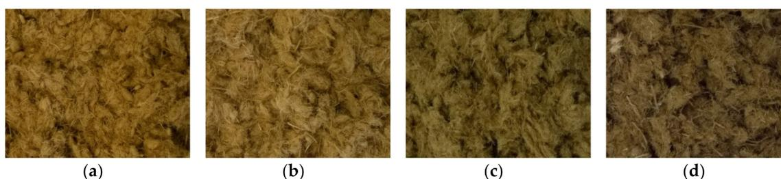
**Figure 8.** Morphology of MDF sample A after steam refining using different treatment conditions [ $\log R_0$ ; °C; min]: (a) 2.47; 150; 10, (b) 3.06; 160; 20, (c) 3.36; 180; 10, (d) 3.95; 190; 20.
