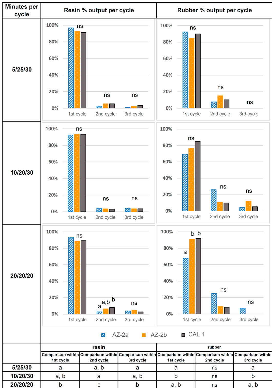
Figure 2. Testing the 3 different cycle schemes in a total extraction time of 60 min for resin extraction and then a total extraction time of 60 min for rubber. Gravimetric yield for resin and rubber in each single stage from the total extracted. Comparisons were made between 2 accessions (AZ-2 and CAL1), with the AZ-2 accession originating from two different plots (AZ-2a and AZ-2b). Different letters in the graph denote significant differences between accessions (AZ-2a, AZ-2b, and CAL1) within cycles, while different letters in columns of the table below denote significant differences between extraction time within the same extraction cycle, both at a 95% level of confidence. ns = non-significant.
