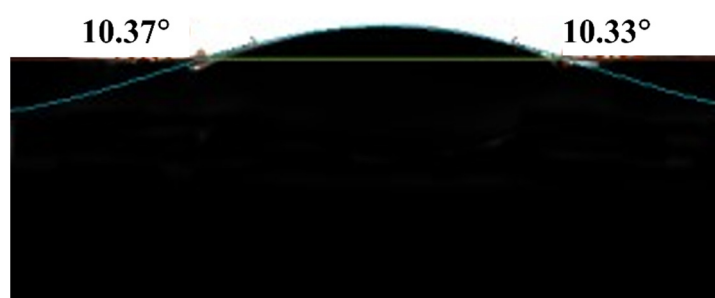
Figure 5. Water contact angle measurement of the HTO/CA.
