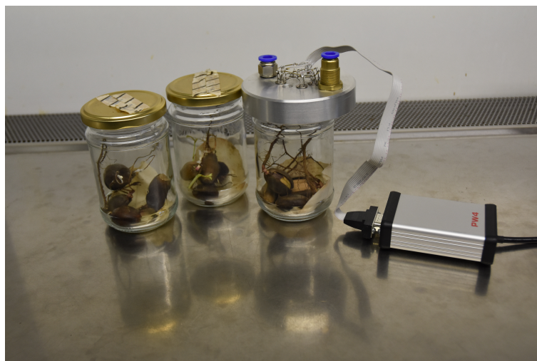
Figure 3. Electronic nose device with measured samples of healthy and infected acorns in jars.
