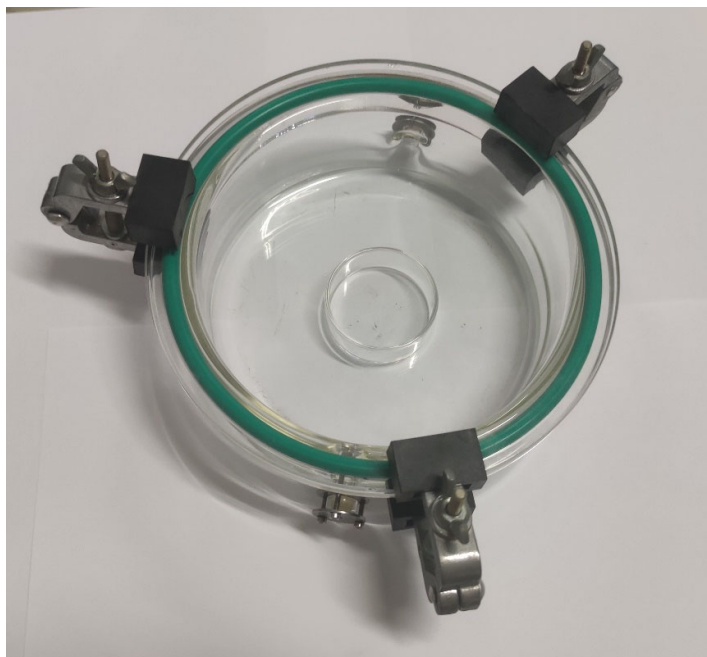
Figure S5 The reaction cell used for isopropanol degradation experiments.
