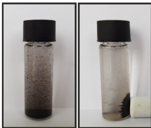
Figure 7. Recoverability of Fe 3 O 4 -CWH nanocatalyst with external magnet.
