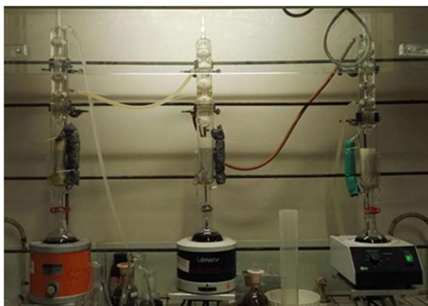
**Figure S2.** Soxhlets assembled in parallel to extract SCH with chloroform and, in a second time, also SCO.
