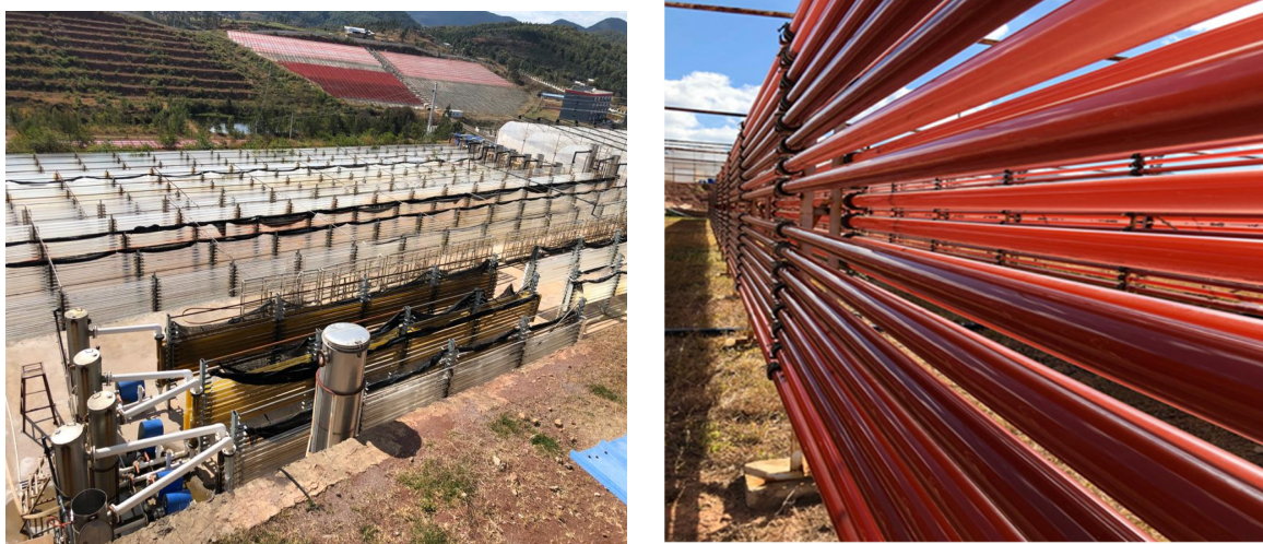
Figure 4. Closed tube bioreactor algae production facility in Yunnan Province, China (Courtesy: Nicholas Cheong, Nova Laboratories Sdn. Bhd.).
