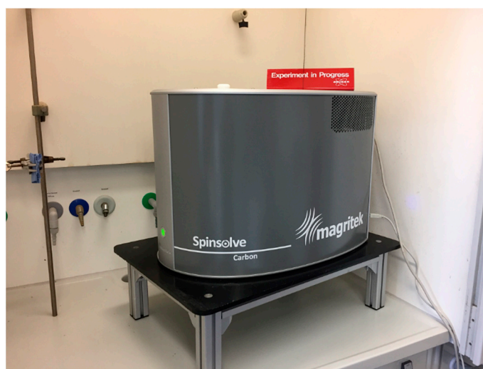
Figure 7. Photo of the utilized Spinsolve placed inside a fume hood in a chemistry laboratory.
