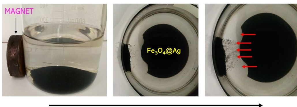
Figure 5. Magnetic properties of the obtained \text{Fe}_3\text{O}_4@Ag particles.
