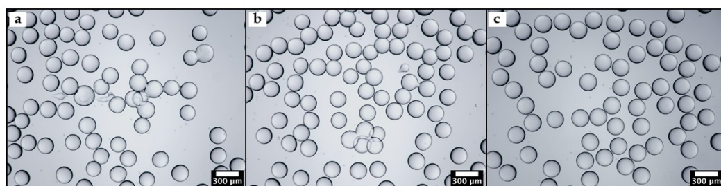
Figure S1. Optical microscopy images of generated PEGDA-99 droplets produced using different concentrations of Xiameter™ RSN-0749 in silicone oil: (a) 2 wt%; (b) 3 wt%; and (c) 3.5 wt%. The droplet diameter was 107 μm in all images.
