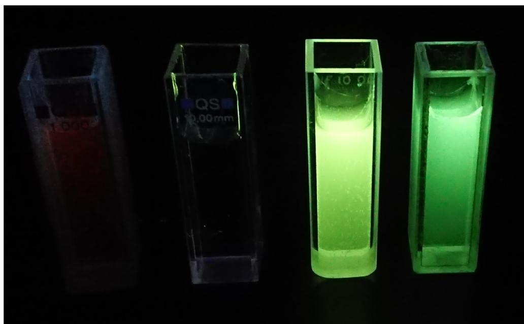
**Figure 8.** Fluorescence color of compound **11a** in MeCN/water mixture (from left to right: 0% 50%, 80% 97% of water). The picture was taken in the dark upon irradiation with a handheld UV lamp ( $\lambda_{\text{em}} = 366$  nm).
